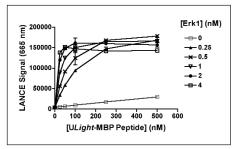
ERK1 enzyme ranging from 0.25 to 4 nM was incubated with the U*Light*-MBP substrate ranging from 25 to 500 nM in kinase assay buffer supplemented with 20  $\mu M$  ATP. Reactions were terminated after 90 min by the addition of EDTA.
